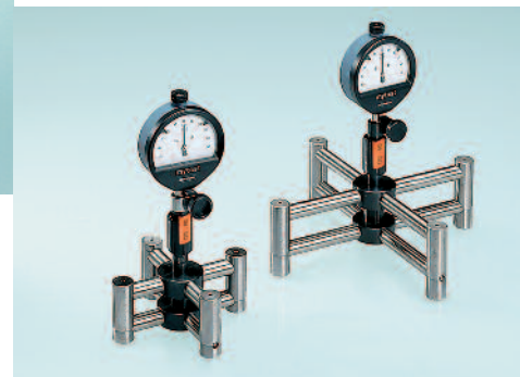
Cross sleeve with runners for dia. 130-800 mm for deep bores or through bores, alignment in the bore is made through the 4 runners
